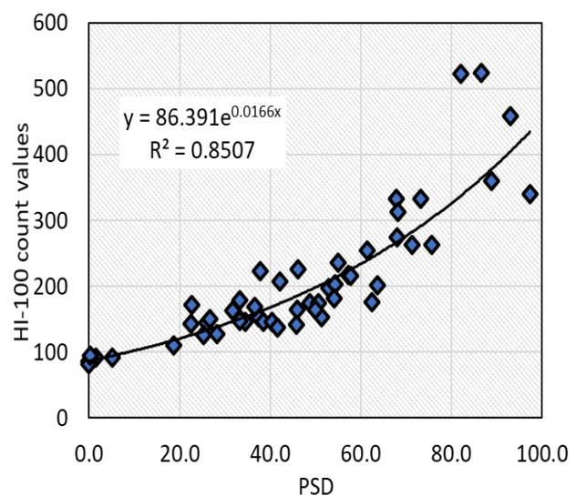
Figure 8(a) Kett HI-100 fitting curve for OPC concrete
