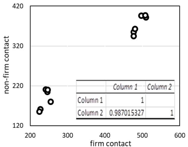
Figure 7(b) Kett HI-100 rubber sensor effects of measuring pressure on count values for 46% PSD and above
