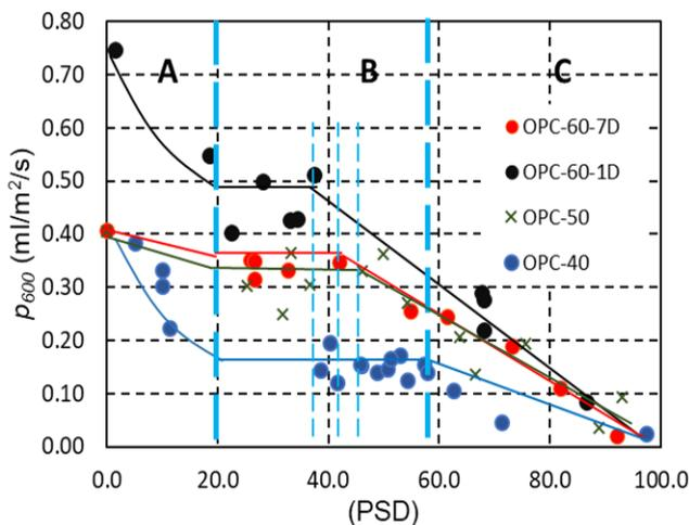
Figure 11 Pattern diagram showing the effects of PSD on surface water absorption
