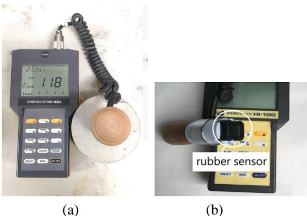
Figure 3 [ (a)Kett HI-100 surface moisture meter
