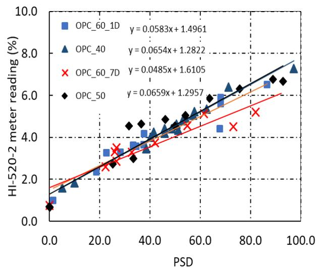
Figure 9(b) Kett HI-520-2 fitting curve for OPC concrete considering water/cement ratios
