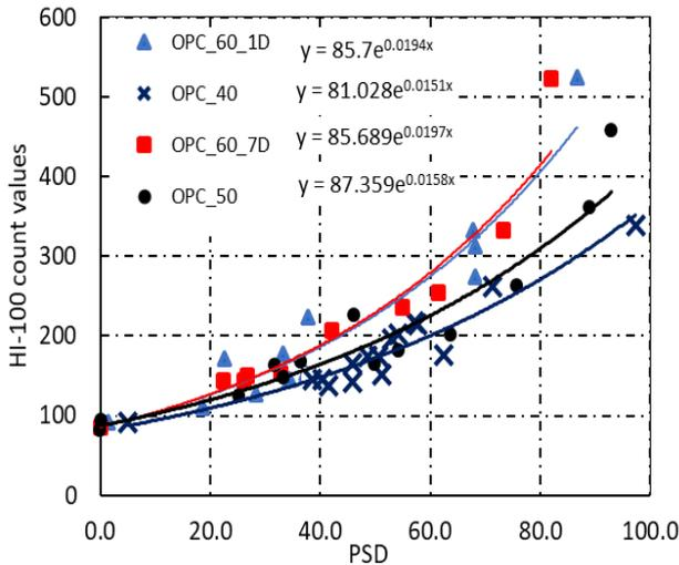
Figure 8(b) Kett HI-100 fitting curve for OPC concrete considering water/cement ratios
