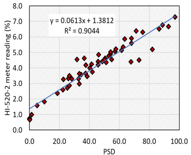
Figure 9(a) Kett HI-520-2 fitting curve for OPC concrete
