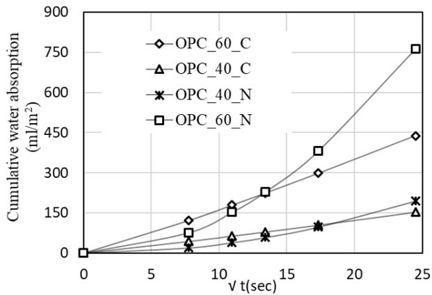
Figure 2 Cumulative water absorption of concretes with and without internal moisture gradient
