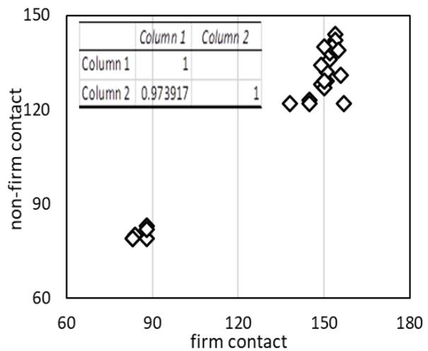
Figure 7(a) Kett HI-100 rubber sensor effects of measuring pressure on count values for 45% PSD and below
