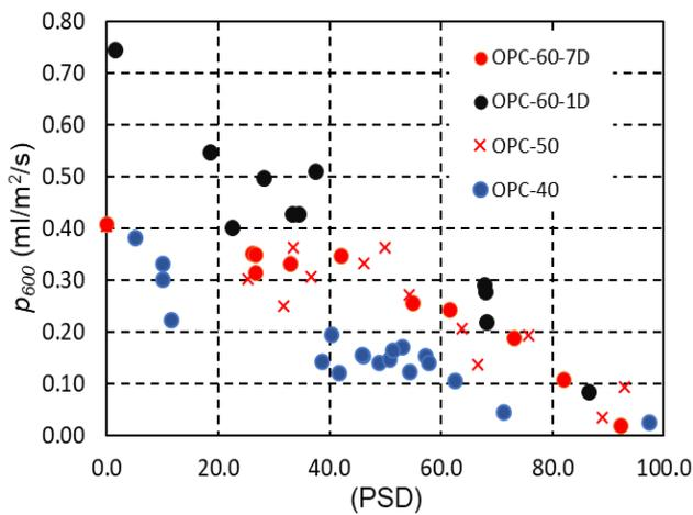
Figure 10 Relationship between PSD and surface water absorption
