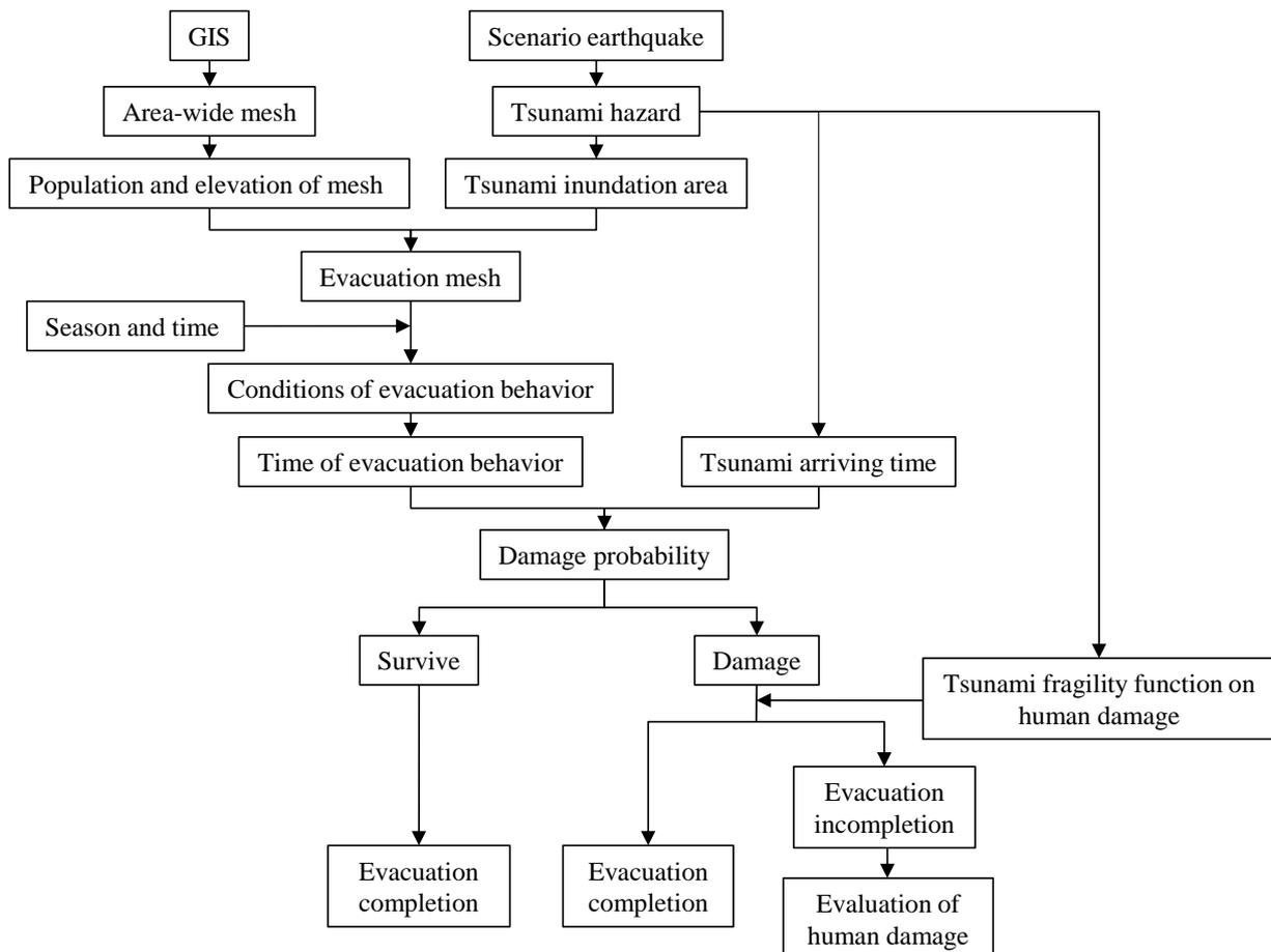
Figure 2.1 Evaluation flow of human damage
