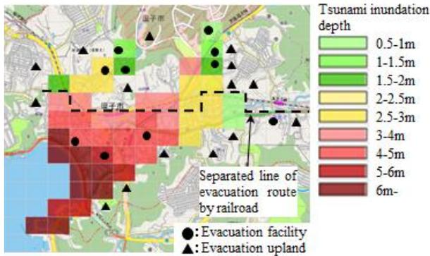
Figure 4.1.2 Tsunami inundation depth
