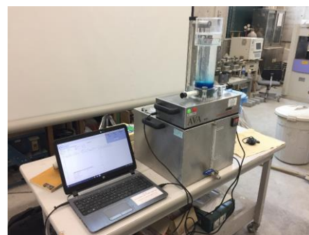
Fig.5 Equipment for air void analysis (AVA)
