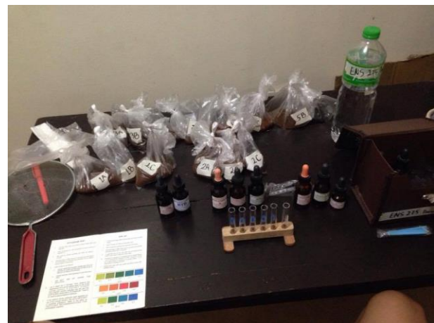
Figure 2. Soil Samples (in plastic bags) and Contents of the Soil Test Kit
