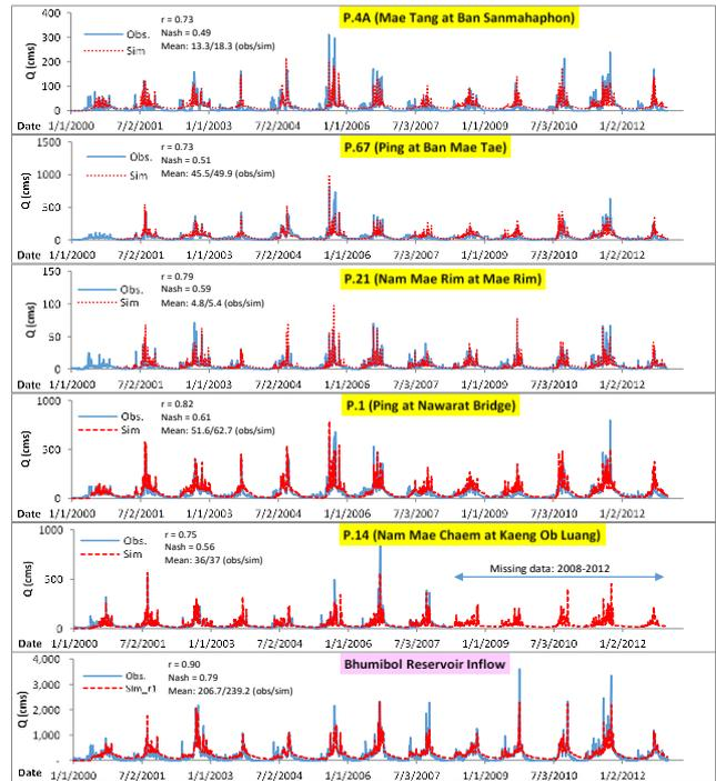
**Fig.2** WEHY hydrology model calibration and validation by comparing the daily mean discharge between simulated and observed flows
