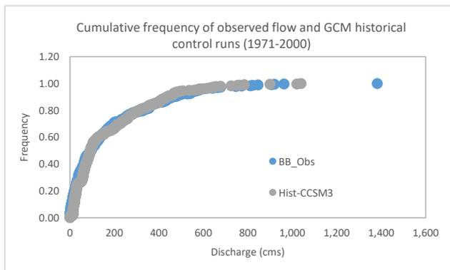
**Fig.4** Comparison of simulated flow based on CCSM3-GCM historical control runs and observed flow at the upper Ping Basin outlet
