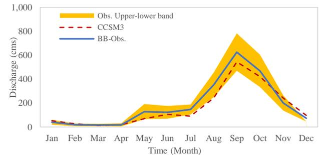
**Fig.5.** Comparisons of mean monthly flow of CCSM3-average flows with the observed flow during 2001-2015, along with 95% confidence band (shade color) of the observed mean monthly flow
