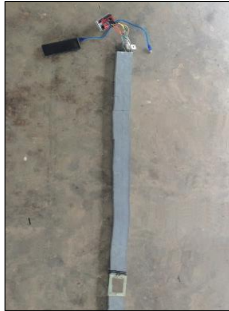
Figure 4: Modified soil moisture sensors.
