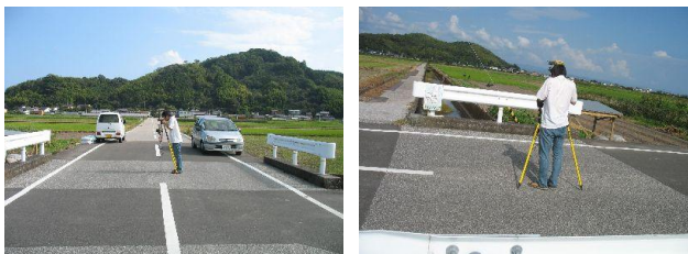
Figure 3.3: Observation scenery of VRS-RTK survey
