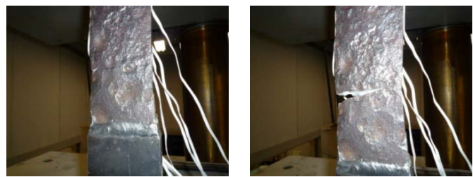
(a) Crack occurring (b) Crack progressing
