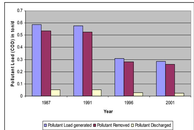
Note: Estimated using 91% removal efficiency of COD by Clean Lake Suwa (Toyoda WWTP) which has operated since 1979
