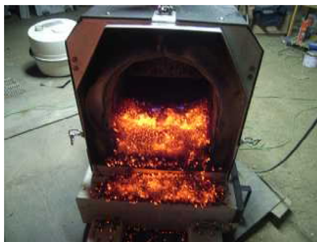
Picture 2. After the combustion of bamboo pellet B
