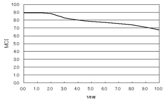
**Figure 11. MCI deterioration forecast**
