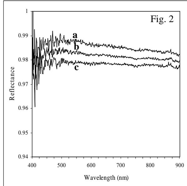
**Figure 2.** Reflectance measurement of reference Panel with different sensor height above the water surface, a: 1.2 meter above the water surface b: 0.5 meter above the water surface c: 1 meter above the water surface
