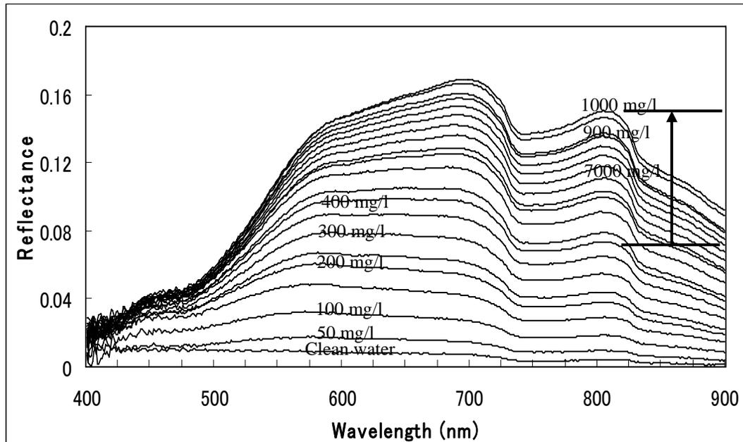
**Figure 5:** Spectral reflectance of water with varying concentration of clayey red soil
