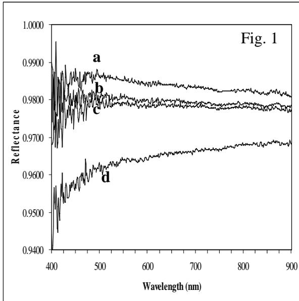
**Figure 1.** Reflectance measurement of reference panel with different warm up time after the spectroradiometer was turned on, a: After 90 minute b: After 120 minute c: After 150 minute d: After 10 minute
