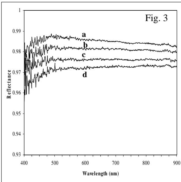
**Figure 3.** Reflectance measurement of reference panel with different cable positions, a: one twist in cable b: zigzag cable c: Straight cable d: many twist
