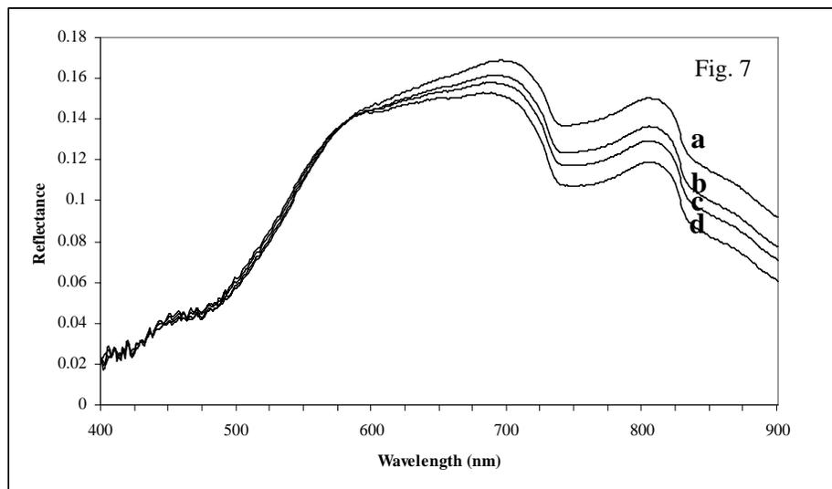
**Figure 7.** Spectral reflectance of water with constant concentration of clayey red soil (1000 mg/l) a: Spectral reflectance after manual mixing 1000mg/l clayey red soil b: spectral reflectance after 1 minute c: Spectral reflectance after 2 minutes d: Spectral reflectance after 3 minutes
