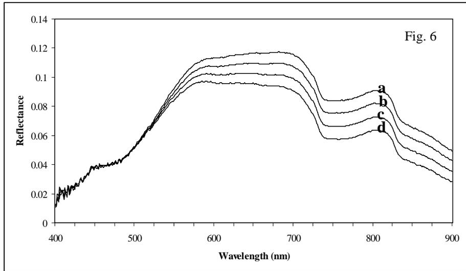
**Figure 6.** Spectral reflectance of water with constant concentration of clayey red soil (500 mg/l) a: Spectral reflectance after manual mixing 500mg/l clayey red soil b: spectral reflectance after 1 minute c: Spectral reflectance after 2 minutes d: Spectral reflectance after 3 minutes
