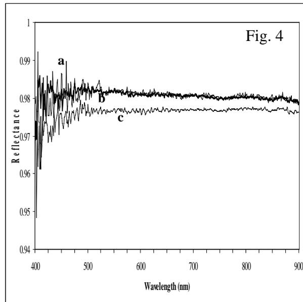
**Figure 4.** Reflectance measurement of reference panel with different illumination angle; a: 60 degree b: 30 degree c: 45 degree
