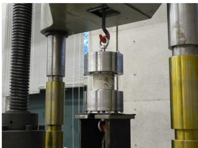
**Fig. 11** Chuck type of tensile testing apparatus
