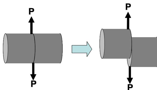
**Fig. 12** Concept of direct pure shearing apparatus:
