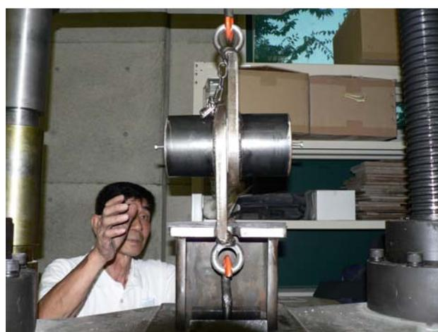
**Fig. 13** Direct pure shearing testing apparatus: not
