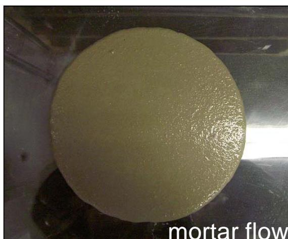
**Fig. 8 Flow of self-compacting mortar of around 300 mm**
