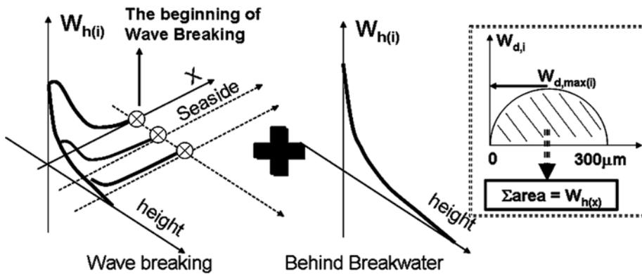
**Fig.1.** Superposition method for aerosol chlorides formation with height, distance and particle sizes distribution ( $d_i = 0\text{-}300 \mu\text{m}$ ) by wave breaking and breakwater
