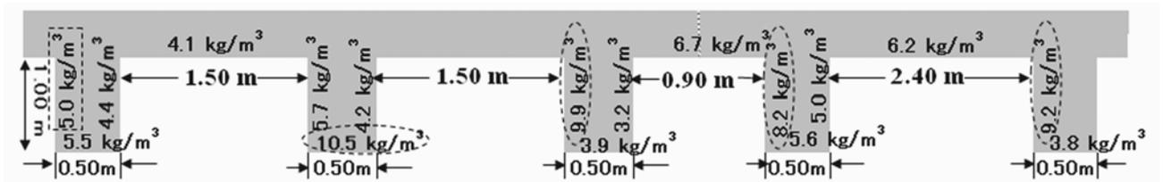
Fig.4. Structural monitoring on surface chloride contents of Ananai Bridge ( $\text{kg/m}^3$ ) after 37 years
