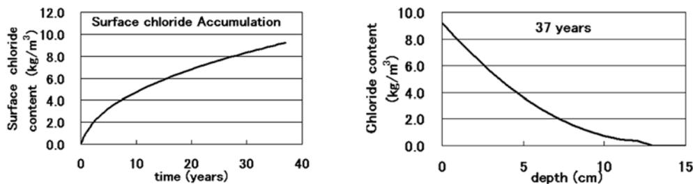
Fig.3. Estimated surface chloride concentration and chloride distribution ( $\text{kg/m}^3$ ) at 37 years simulation
