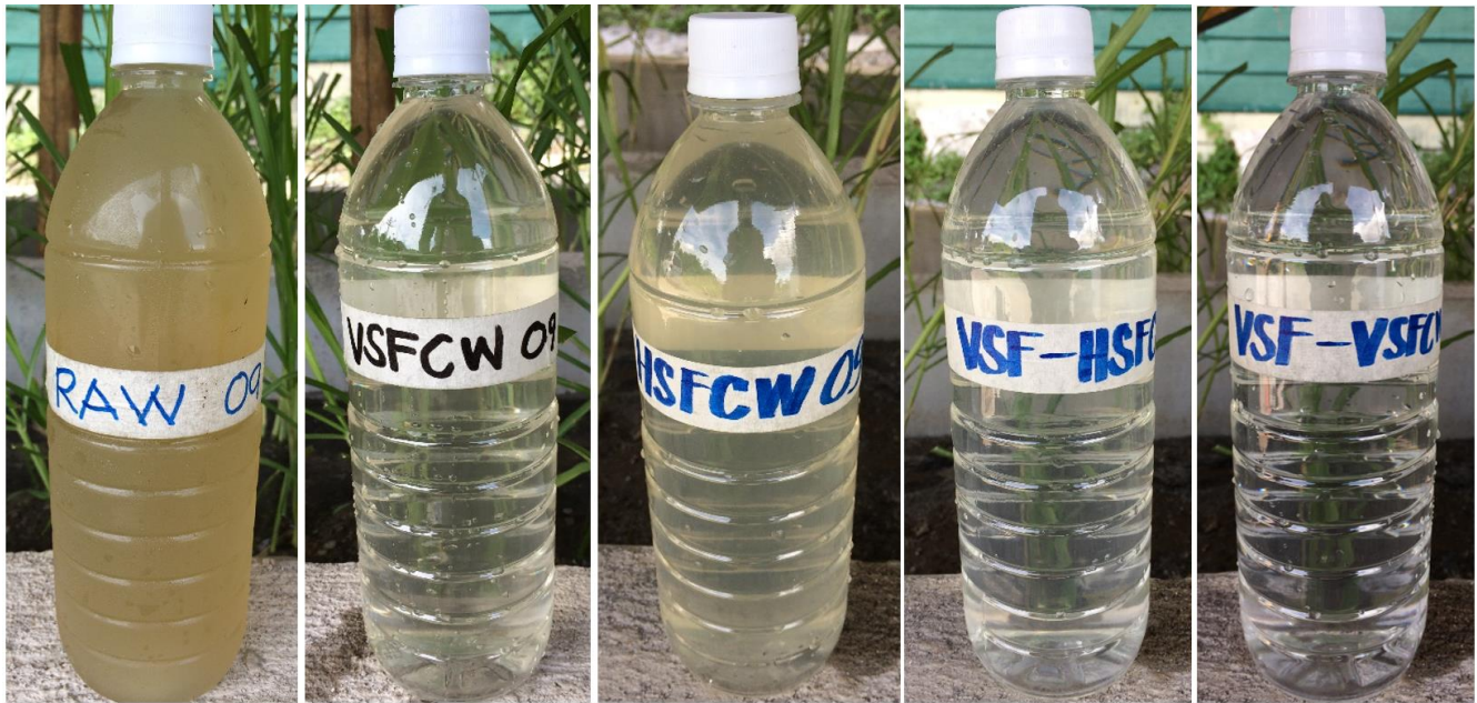
Figure 3. Raw wastewater (RAW), Vertical (VSFCW), Horizontal (HSFCW), Vertical in Series (VSF-VSFCW), and Hybrid (VSF-HSFCW) Effluent samples
