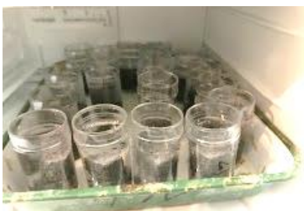
Figure 1 Photo of small-sized samples during scaling test
