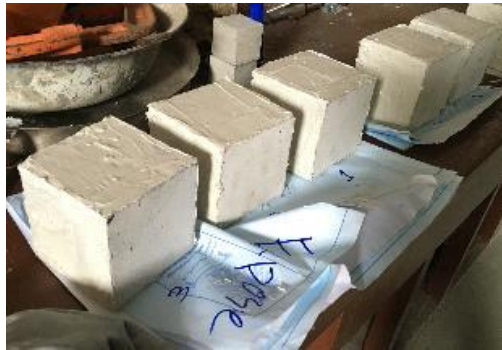
Figure 2.13 the mortar specimens coated with epoxy
