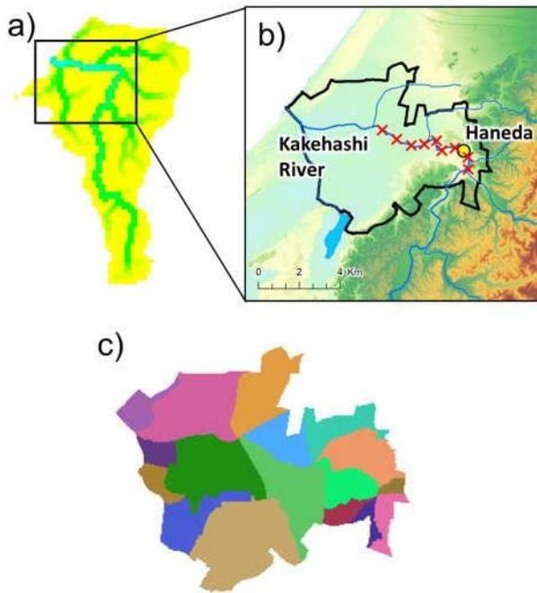
Figure 2 (a) Simulation area of RRI model, (b) Simulation area of inundation simulation (indicated by black line). Red crossed indicate sections of dyke break. (c) drainage districts for inundation simulations.
