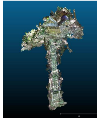
Figure 2.9 The obtained point cloud by SfM
