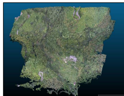
Figure 2.7 The point cloud obtained by SfM from UAV
