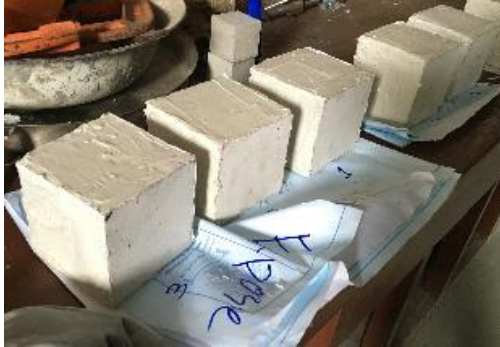
Figure 2.13 the mortar specimens coated with epoxy
