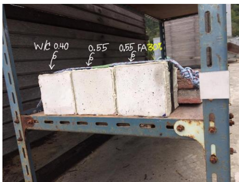
Figure 2.15 On-site exposure set
