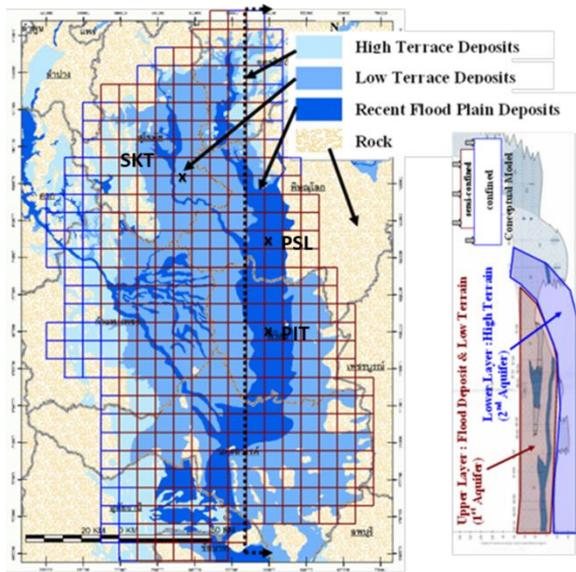
Figure.2 Layer aquifer's conceptual model and model grid design
