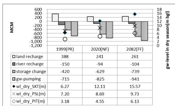
Figure 7 The annual flow of groundwater system (aquifer 1) and gw-level in dry season of SKT and PSL in the drought years (like 1999, 2020 and 2082)
