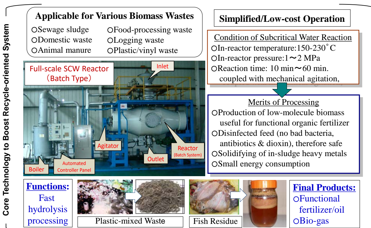
Figure A-1 Technological and Operational Characteristics of Subcritical Water Reactor (Batch-type)
