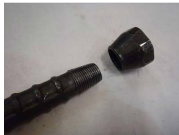
Figure-5 Taper shaped screw mechanism
