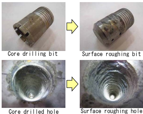
Figure-3 Inner surface roughing of drilled hole
