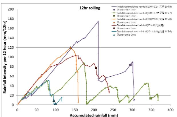
Figure 8 Analysis results of “Snake Line” model based on different time rolling rainfall intensities
