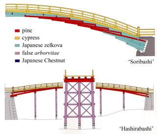
Figure 2.3 Timbers for structural members
