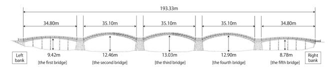
Figure 2.2 Dimensions of each part
