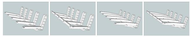
Figure 4.10 Reproduction of the bridge construction process ('Soribashi')
