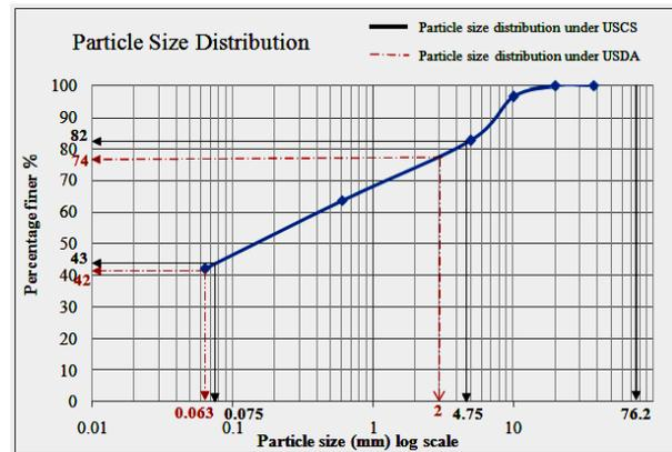
Figure 1. Particle size distribution according to USCS and USDA
