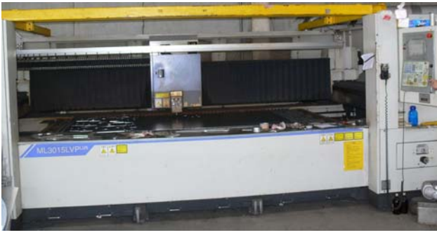
Photo 3.1.1 Mitsubishi laser cutting machine (3500W ML3015LVPlus)
