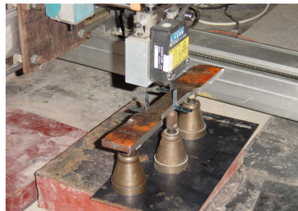
Photo 1: Condition of thickness measurement
