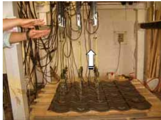
Figure5 roof tile pulling-up test device (Okada and Kikitsu, 2005)
