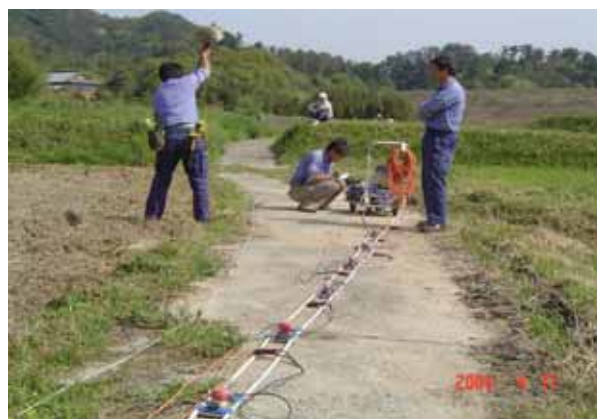
Fig. 3 Operation of the surface wave prospecting at Tanaka site
