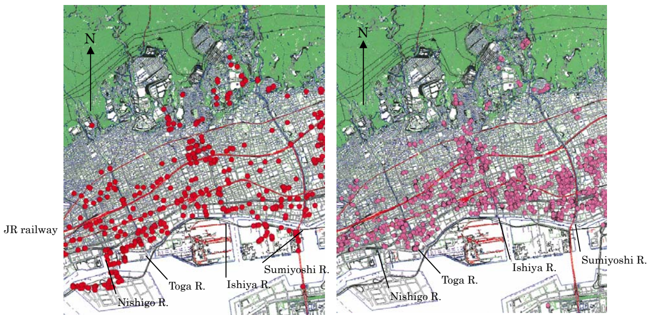
Fig. 2 Damaged points of a) water and b) sewage.
