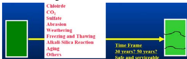
Figure 1. Environmental Loadings on Concrete
