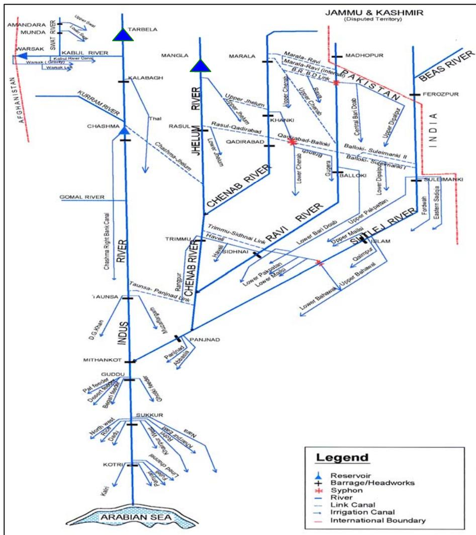
Figure 1: Schematic diagram of Indus Basin Network
