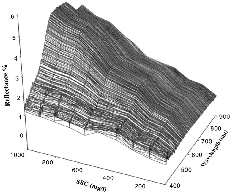
Figure 3. Spectral Reflectance of Water With Varying Concentration of Collected Soil Sample
