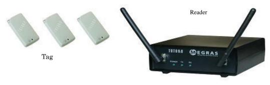
Figure 4 RFID tags and Reader
