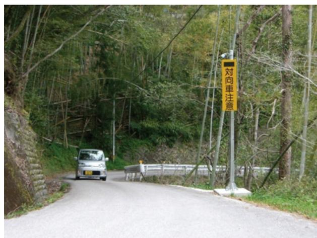
Fig5 Simplified type (fixed display board + LED)
