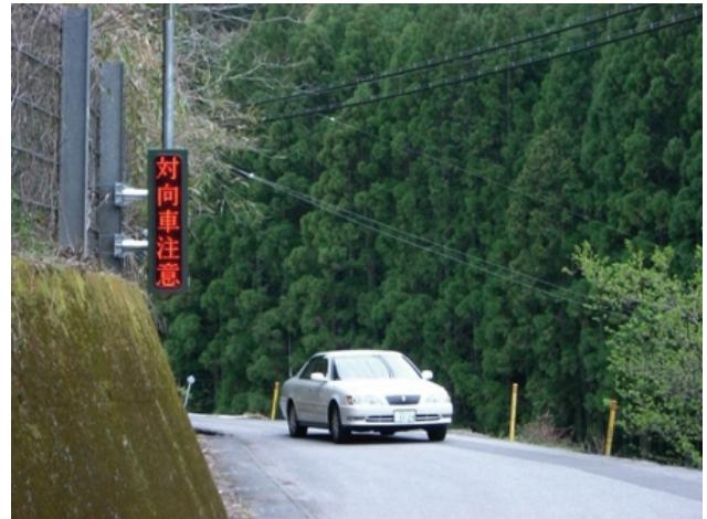
Fig4 Standard type (LED display board)
