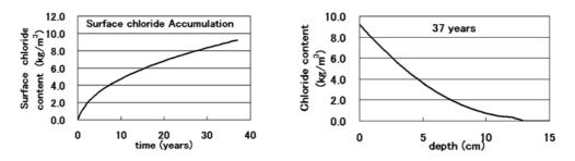
Fig.3. Estimated surface chloride concentration and chloride distribution (kg/m<sup>3</sup>) at 37 years simulation
