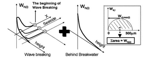
**Fig.1**. Superposition method for aerosol chlorides formation with height, distance and particle sizes distribution ( $d_i = 0.300 \ \mu m$ ) by wave breaking and breakwater
